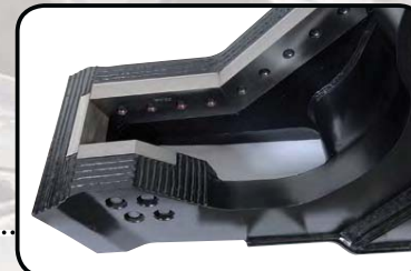
All New Blades All the blades have been redesigned in a rhomboid shape to reduce stresses on the jaws. Each main blade can be turned effectively 3 times The new blades are threaded for easier removal and installation.
