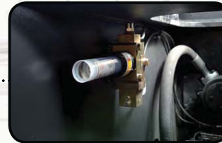
New Manto-Autolube System® All of the largest shears are equipped with the "Manto-Autolube", a unique total shear greasing system, ensuring all moving parts are regularly greased.
